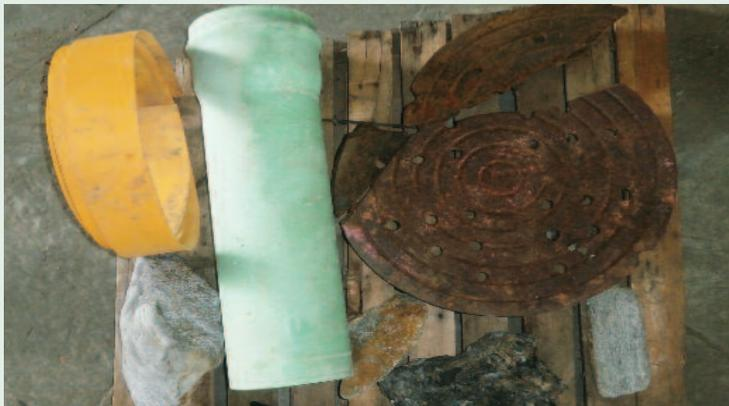
MWA crews needed two days to remove this construction debris from a blocked sewer line. The Authority determined this caused a recent major sewer spill near the Ocmulgee River.
