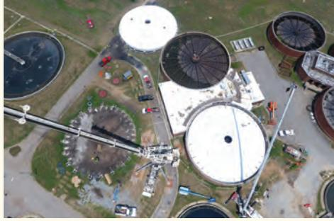
The MWA is investing over \$40 million to renew and rehabilitate its two water reclamation facilities. The new digester lids (pictured) at the Lower Poplar Plant are among the many facility upgrades.
